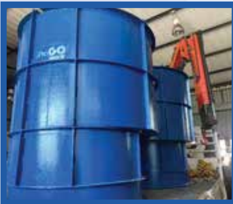
Cyclone fabricated from Chrome carbide material
