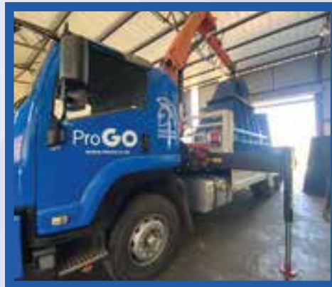
Cyclone fabricated from Chrome carbide material
